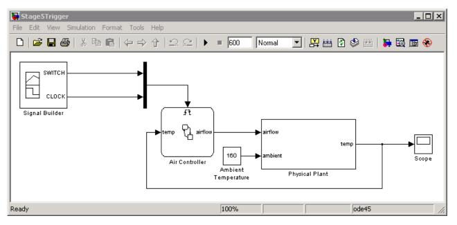
The output signal of the Mux block connects to the input trigger port of the Stateflow block. Your chart should look like this:
