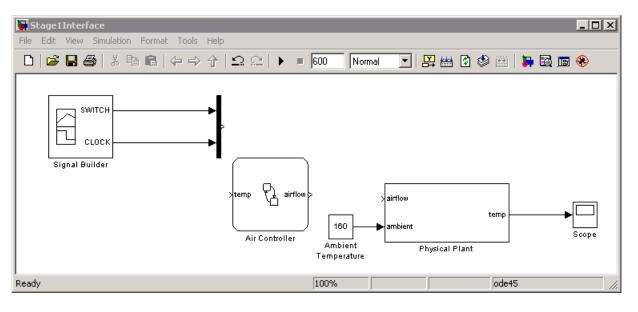
Notice that the input temp and output airflow have been added to the Stateflow block:
