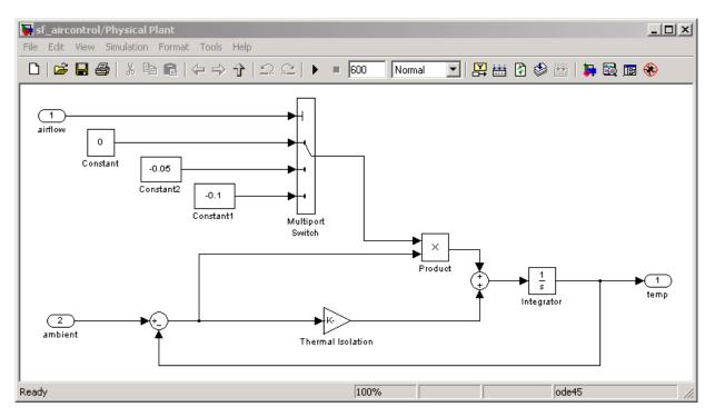
In this model, the internal temperature of the plant attempts to rise to achieve steady state with the ambient air temperature, set at a constant 160 degrees (as shown in "How the Stateflow Chart Works with the Simulink Model" on page 2-6). The rate at which the internal temperature rises depends in part on the degree of thermal isolation in the plant and the amount of cooling activity.
